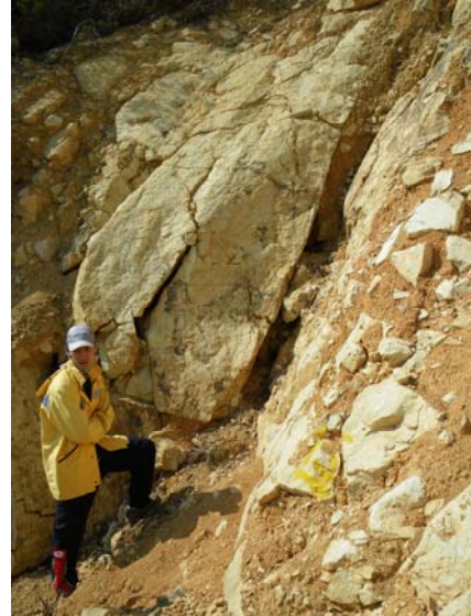
(b) Open and infilled discontinuities at landslide scarp of the main source of the June 2008 Shek Mun Kap debris flow
