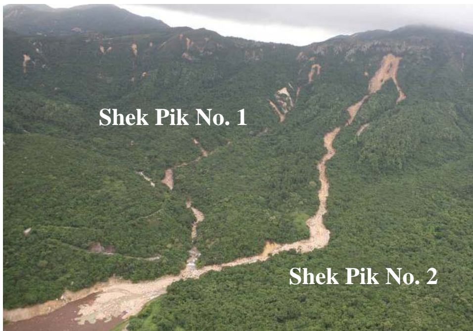
Figure 19: Large debris flows on Lantau in the June 2008 rainstorm (Note: Shek Pik No. 1 and No. 2 debris flows are shown; see Figure 5 for debris flows in the area in November 1993)
